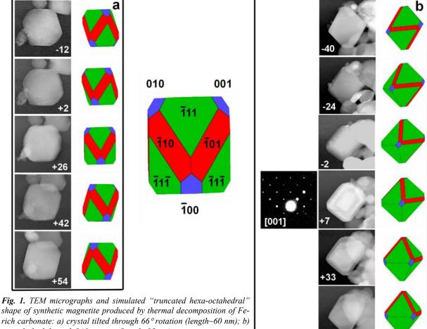
shape of synthetic magnetite produced by thermal decomposition of Ferich carbonate: a) crystal tilted through 66° rotation (length~60 nm); b) crystal tilted through 84° rotation (length~85 nm).
