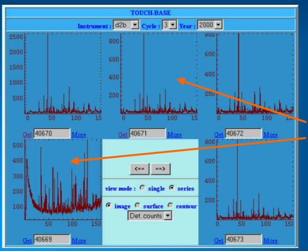
Series of D2B powder diffraction patterns
