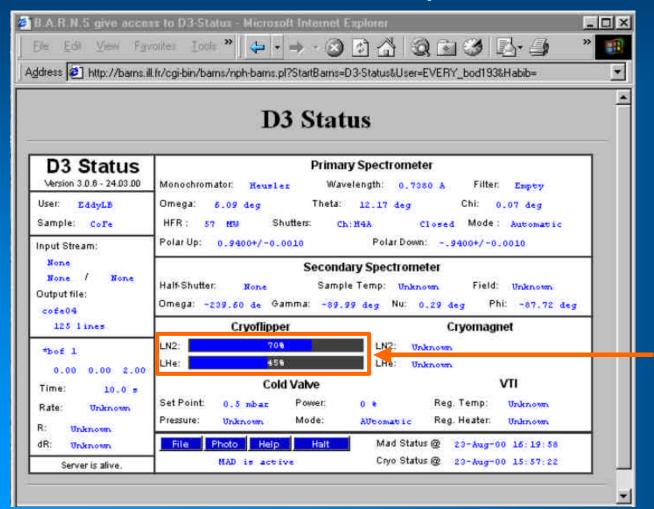
Java graphic monitor for cryogenic levels, temperature etc
