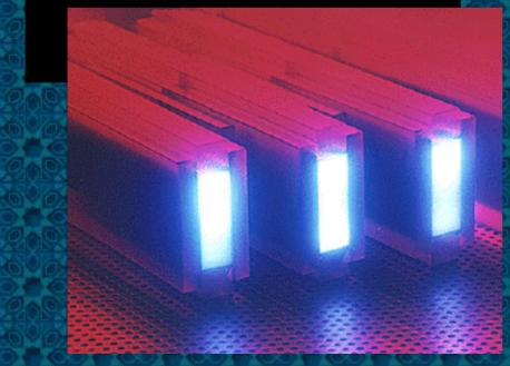
I "Neutron guide tubes" bring the neutrons to the experiment
