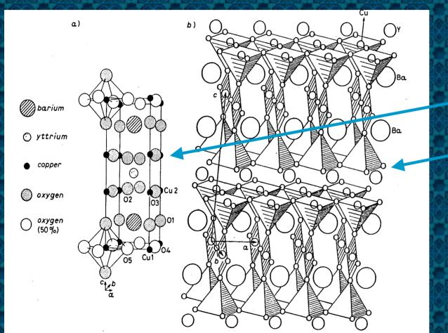
The 90K high Tc superconductor I Left -by X-rays
