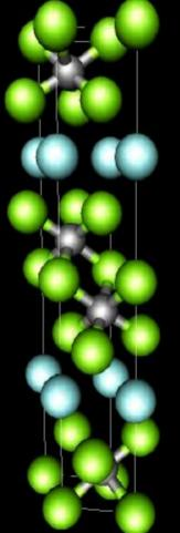
Titanium silicon carbide Ti<sub>3</sub>SiC<sub>2</sub> conducts heat and electricity I It is tough, easily machinable I Potential engineering applications as a light replacement for metals
