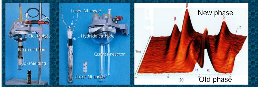
Neutrons penetrate deep inside batteries during charge-discharge cycle
