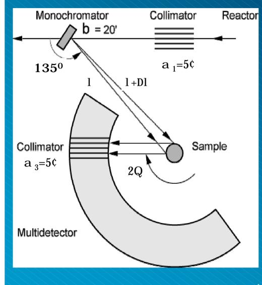
A "white" beam of neutrons from the reactor is collimated
