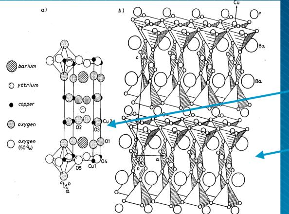
The 90K high Tc Superconductor Y<sub>1</sub>Ba<sub>2</sub>Cu<sub>3</sub>O<sub>7</sub>
