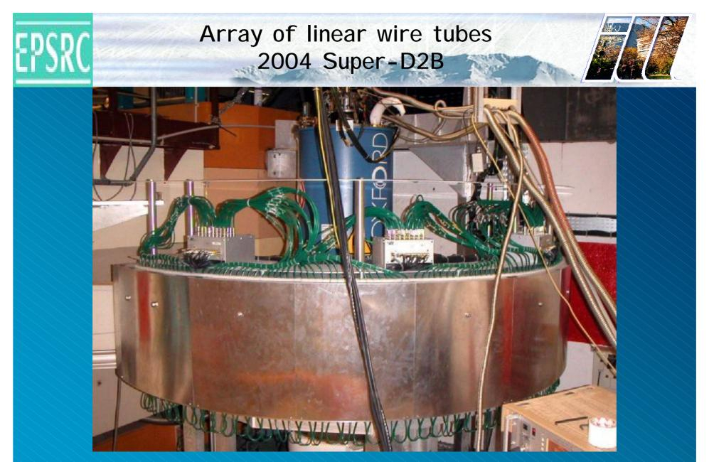
Completed 300 mm high 2D-detector, with 6 Tesla cryomagnet
