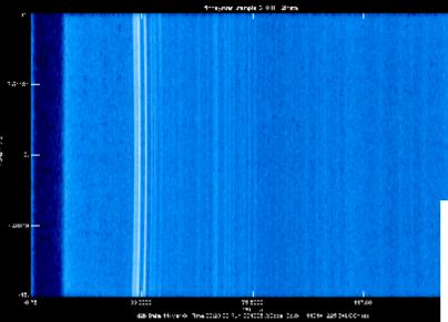
180 mg I ce sample measured at high pressure and 80K in the D2B displex (J. Finney, E.Suard)
