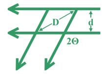
Fig. 11 For angles near  $90^{\circ}$  with a radial collimator, scattering would be limited to a small volume of diameter D.
