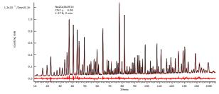
Fig. 6 The complete refined diffraction pattern obtained from Na<sub>2</sub>Ca<sub>3</sub>Al<sub>2</sub>F<sub>14</sub> in only 2 minutes on D20 in high resolution mode.
