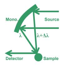
Fig. 10 Focusing of a large band of wavelengths still permits high resolution at high monochromator take-off angles.
