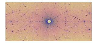
Fig. 3 The image-plate detector and high flux on the sample allow surveys of reciprocal space eg this quasi-crystal on LADI.
