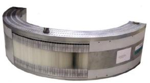
Fig 13. The Dracula radial collimator will cover a very large solid angle  $(160^{\circ}x30^{\circ}$  vertical) yet restrict scattering to a very small volume of diameter ~5mm around the sample. It will be similar to the new D20 radial collimator above (EuroCollimators, 2005).
