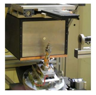
Fig. 4 Orient Express at ILL is a simple CCD detector on a continuous white neutron beam (Ouladdiaf, this conference).
