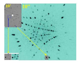
Fig. 5 Diffraction pattern from a small ruby crystal obtained on Orient Express in 10 seconds, instead of 10 minutes with film.
