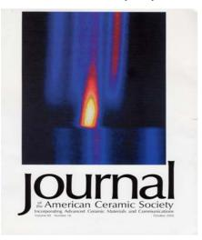
Fig. 7 The explosive SHS reaction in  $Ti_3SiC_2$  on D20. The intermediate phase (bright spot) lasts only ~1 second.
