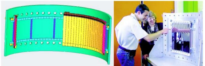
**Fig. 6.** The new 30°x120° 2D-PSD for D19. Large detectors match the solid angle of the best pulsed-neutron diffractometers, while benefiting from the very high flux available on the sample at a reactor source. (Guerard et al. 2002).
