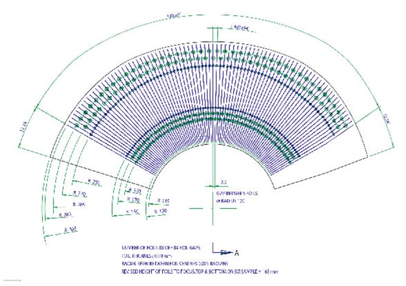
**Fig.5.** The Dracula radial collimator will cover a very large solid angle  $(160^{\circ} \times 30^{\circ} \text{ vertical})$  yet restrict scattering to a very small volume of diameter ~5mm around the sample. (EuroCollimators Cheltenham, 2003).
