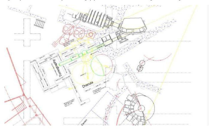
**Fig. 1b** Option B: Dracula would displace the tomography station on the 200mm diameter high flux H9 Lohengrin beam tube. The H9 beam tube is perhaps the most intense thermal neutron beam anywhere, and if we are to compete with the American pulsed source this position must be used to maximum advantage.
