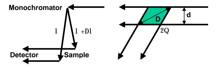
Fig. 2(a) Mosaic monochromator focussing a wide band of wavelengths 2(b) Small scattering volume with a radial collimator.
