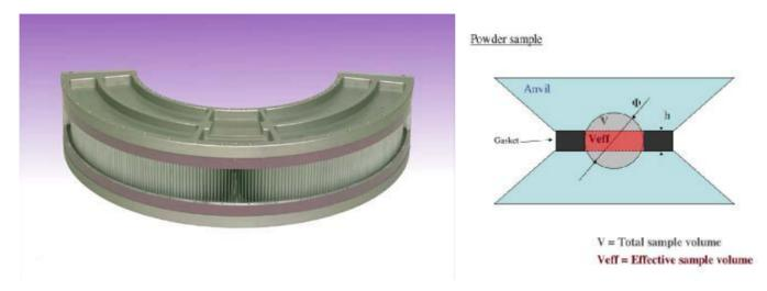
Fig. 4 Radial collimator of the type to be used for Dracula 2(b) High pressure Paris-Edinburgh cell being constructed for ILL.
