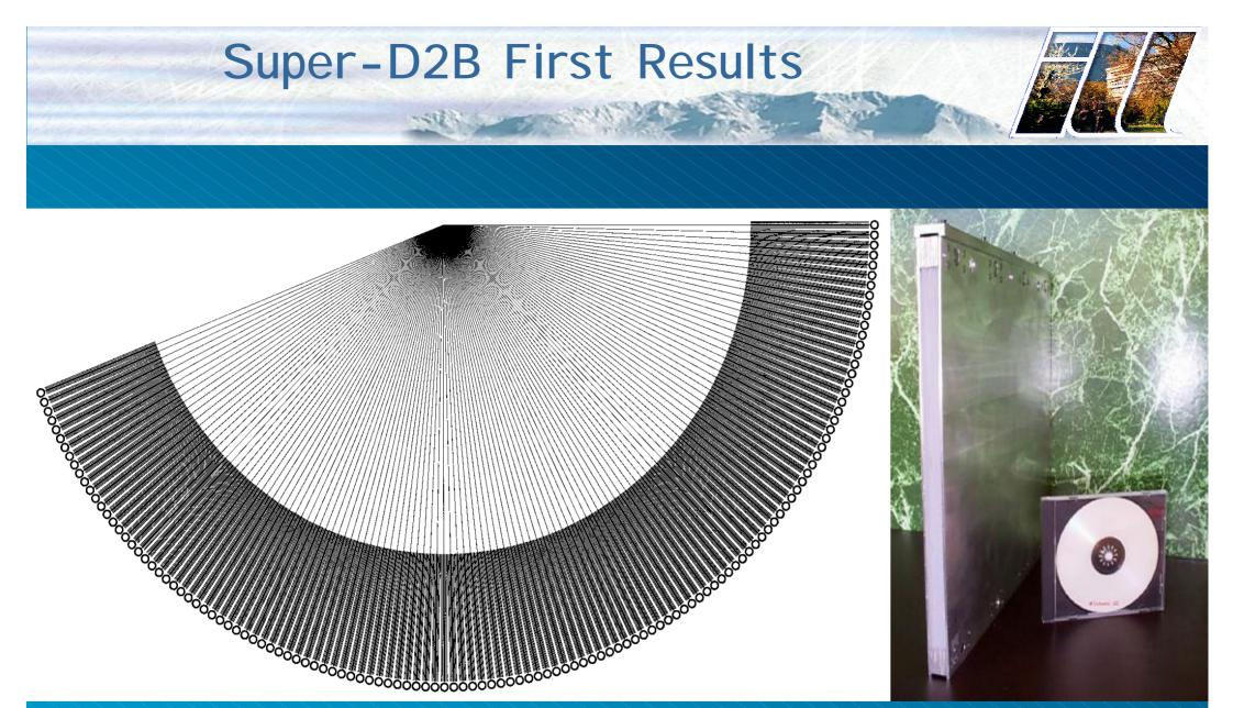
•128 x 300 mm high resistive wire detectors, high resolution collimators
