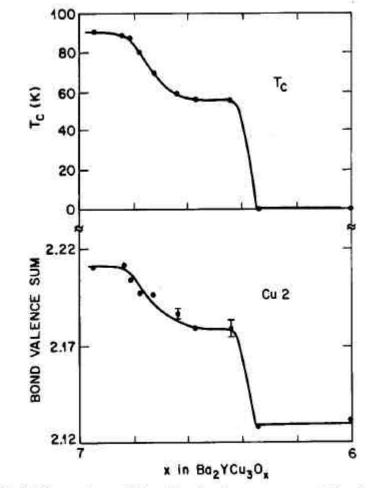
Fig. 16. Comparison of  $T_c$  and bond valence sum around the plane copper as a function of oxygen stoichiometry.
