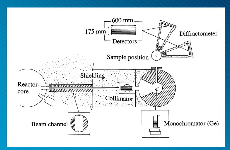
The liner wire PSD powder diffractometer at Kjeller, Norway.
