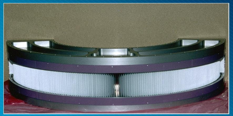
Radial Collimator for new HRPT diffractometer at PSI Zurich (Fast, medium-high resolution machine) Peter Fischer et al.
