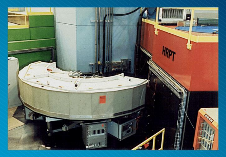
HRPT 1600 cell PSD powder diffractometer at PSI (Zurich)
