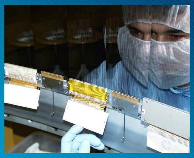
Instead of wires, a printed circuit is used.
