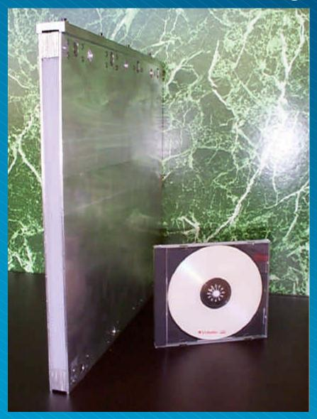
Prototype super-D2B 5' mylar foil collimator
