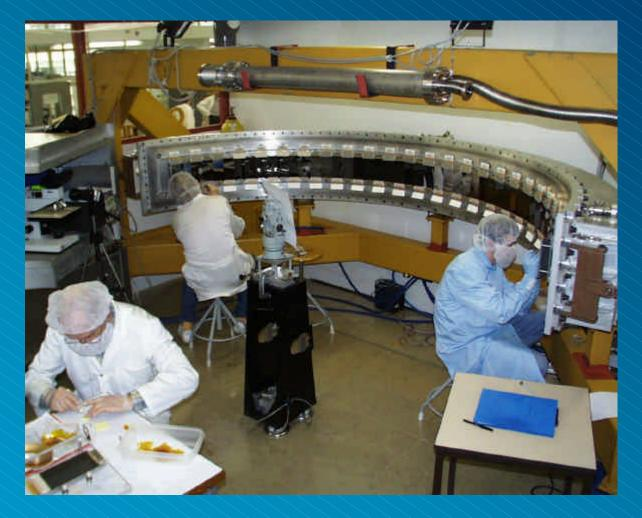
25 plates of 64 electrodes are assembled to produce a 1600-wire detector covering 160°.
