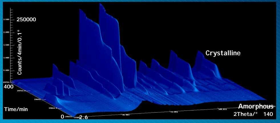
Complete diffraction pattern in minutes or seconds, scan through temperature
