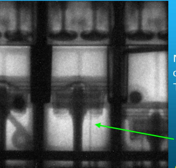
Neutron radiograph of a real BMW engine Time 0.5 milliseconds
