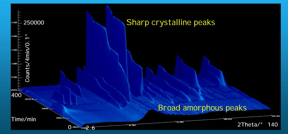
Complete diffraction pattern in minutes or seconds, scanning through temperature R. Cywinski, S. Kilcoyne (St Andrews)
