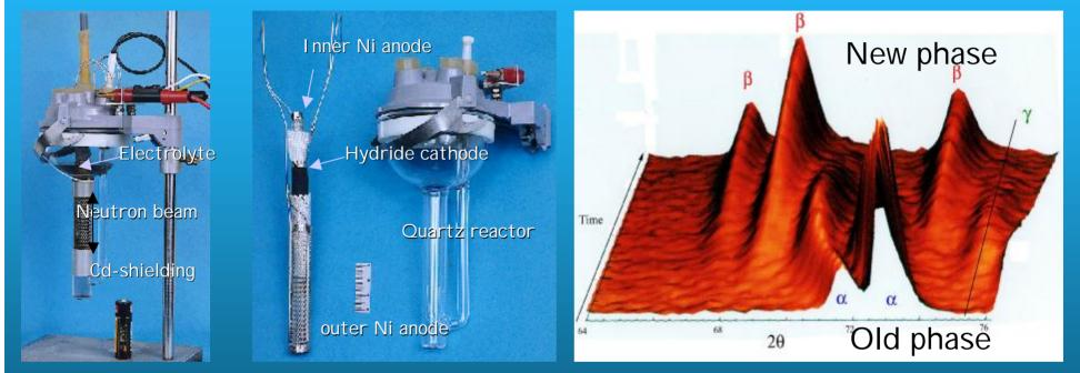
Neutrons penetrate deep inside batteries during charge-discharge cycle
