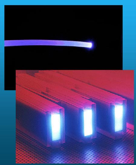
I "Neutron guide tubes" bring the neutrons to the experiment
