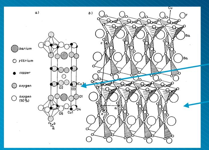
The 90K high Tc Superconductor  $Y_1Ba_2Cu_3O_7$
