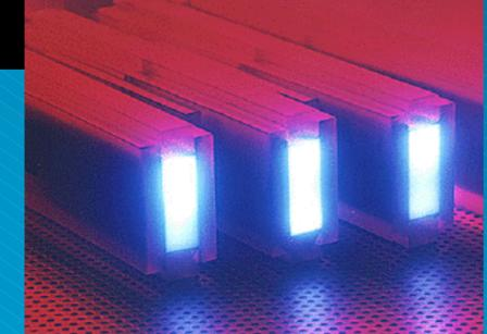
I "Neutron guide tubes" bring the neutrons to the experiment
