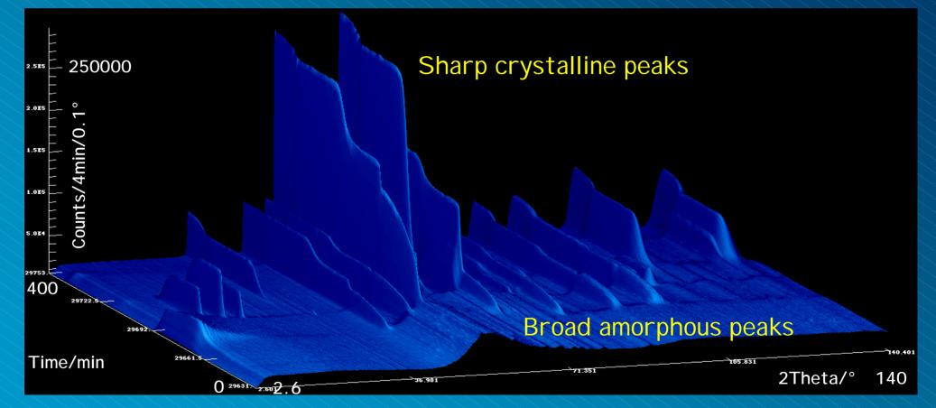
Complete diffraction pattern in minutes or seconds, scanning through temperature
