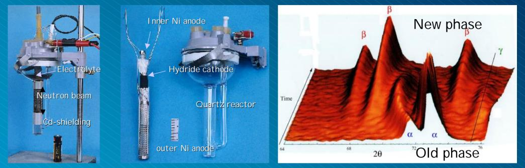
Neutrons penetrate deep inside batteries during charge-discharge cycle
