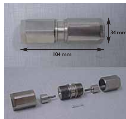
Figure 1: Photographs of the 30 kbar non-magnetic clamp cell designed at the Institute for High Pressure Physics and used in the 10 T cryomagnet on the polarised neutron diffractometer D3.
