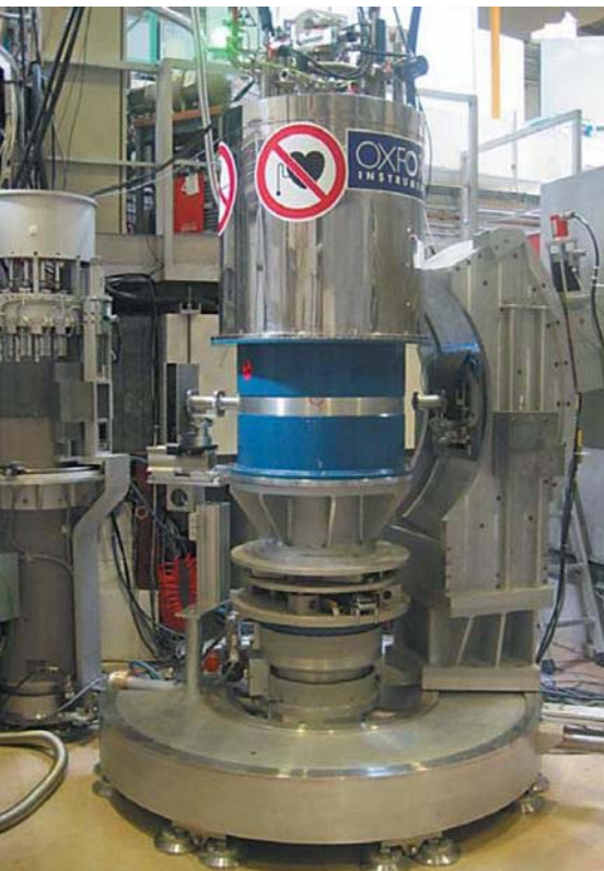
Figure 1: The new D23 secondary spectrometer with the 15 T ILL cryomagnet mounted.
