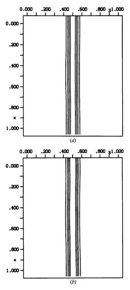
Fig. 2. Section of the four-dimensional Fourier synthesis of  $(LaS)_{1.14}NbS_2$  at the position of the La atom (x = 0 and z = 0.174). Contours are plotted at intervals of 1/5 of the maximum density. (a) Main reflections with phases from the basic structure refinement. (b) Main reflections with phases from the modulated structure refinement.
