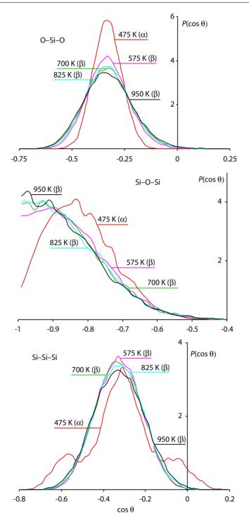
**Figure 7.** Three bond-angle distribution functions for cristobalite at the five temperatures. In each case, the distribution functions for all temperatures in the  $\beta$ -phase are very similar, but significantly different from the distribution functions of the  $\alpha$ -phase. The data are given as functions of  $\cos \theta$ , where  $\theta$  is the particular bond angle in each case.
