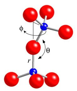
**Figure 8.** Definitions of the angles associated with the relative orientations of two linked SiO<sub>4</sub> tetrahedra.  $\theta$  is the Si–O–Si bond angle.  $\phi$  is the angle between the direction of the tilt of the bridging Si–O bond of one tetrahedron projected onto the plane of the three basal oxygen atoms of the other tetrahedron: the value  $\phi = 0$  corresponds to the bridging Si–O bond tilting in the direction of one of the basal oxygen atoms.
