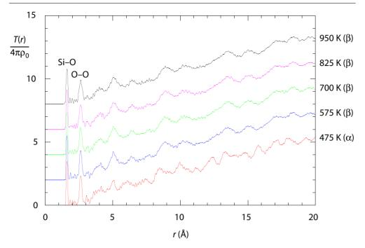
**Figure 3.** Functions  $T(r)/4\pi\rho_0$  for cristobalite at five temperatures, obtained by Fourier transformation of the data shown in figure 2. The two peaks at the lowest distances r correspond to the Si–O and O–O bonds. Data from successive temperatures have been shifted by a vertical offset for clarity.
