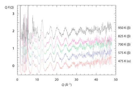
**Figure 2.** Measurements of QF(Q) for cristobalite at five temperatures, with the data from successive temperatures shifted by a vertical offset for clarity. The large scatter of the data at high values of Q arises because of the factor of Q. The sharp peaks at the lower values of Q are the Bragg peaks.
