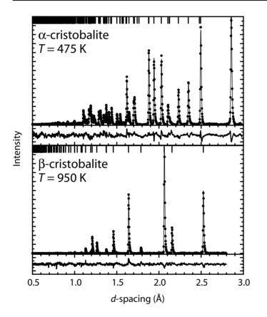
**Figure 4.** Two examples of the Rietveld fitting to the diffraction data. The vertical bars along the top of each plot represent the *d*-spacings of the Bragg peaks. The bottom curve in each case represents the difference between the calculated and experimental diffraction patterns scaled by the standard deviation of each point.
