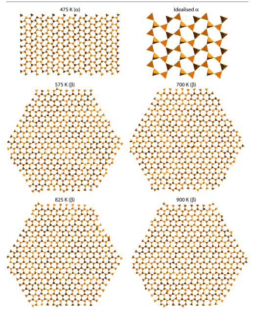
**Figure 5.** Atomic configurations of cristobalite at the five temperatures obtained from the RMC refinement, with the atoms represented as shaded SiO<sub>4</sub> tetrahedra. The views are down the [111] axes of the cubic  $\beta$ -phase, and down the corresponding [201] axis of the tetragonal phase. The figure also shows the corresponding projection of the ideal tetragonal phase with no thermal motion.
