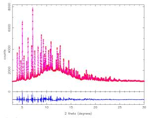
Fig. 2 Final synchrotron X-ray diffraction Rietveld plot for tetracycline hydrochloride.
