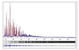
Fig. 3 Final conventional X-ray diffraction Rietveld plot for tetracycline hydrochloride.
